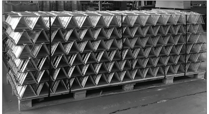
Wire Truss is used to connect the bottom and top concrete layers in a precast “sandwich” panel. Foam insulation is placed between the Wire Truss to create an energy-efficient panel.
