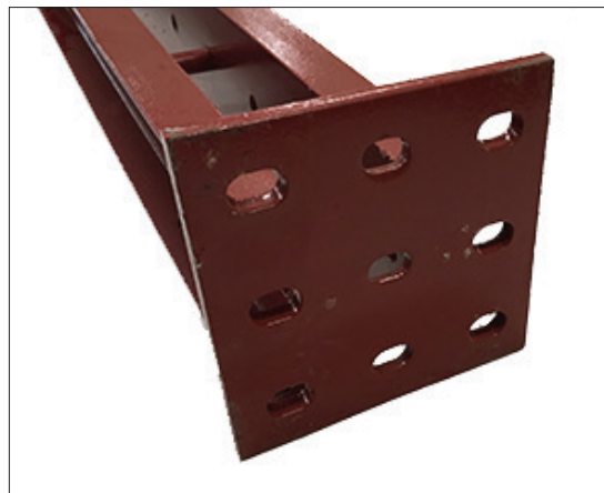
Butt Plate Walers have 1/2"x9"x9" end plates with slotted holes for end-to-end connections.
