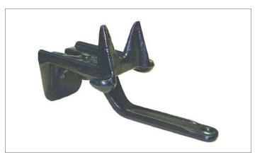
The TieLock Bracket, sometimes called a Camlock bracket, has a pivoting handle that captures the tie loop and 2x4 lumber waler at the same time.
