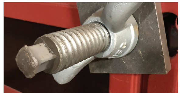
Hitting Taper Ties on the squared end will avoid thread damage and stripping difficulty.
