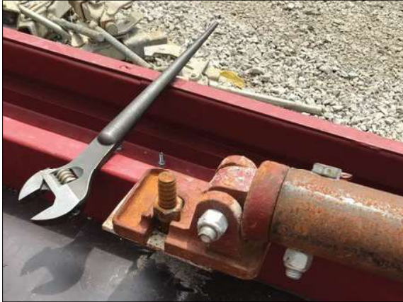
Bracing can travel with each SureCurve gang using the shoe attachment plate.
