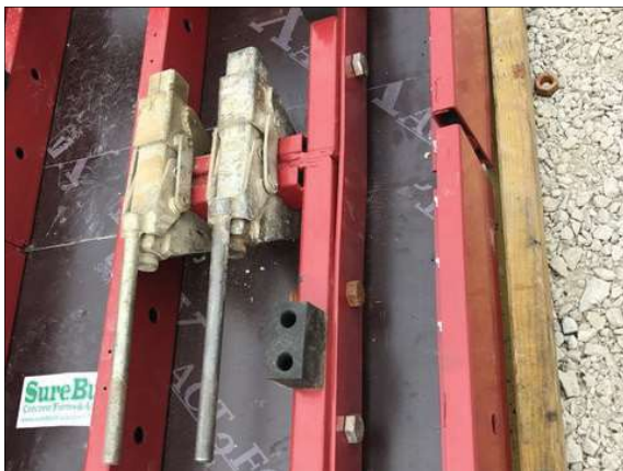
Connecting clamps and stacking plate span the joint between two SureCurve panels.
