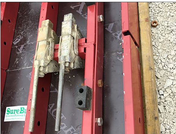
Connecting clamps and stacking plate span the joint between two SureCurve panels.
