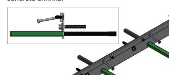
Available with and without square dowels and tube. The opening for the Square Dowel is positioned at mid-slab height.
