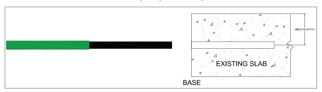
2. Set E2N Square Dowel and Tube in epoxy grout with Tube flush with existing slab and foam on the left and right sides.
