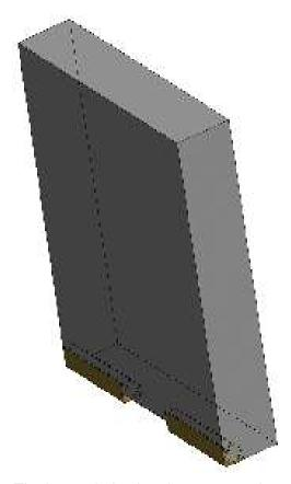
The integral plastic edge protects the concrete when handling and moving tilt-up panels.
