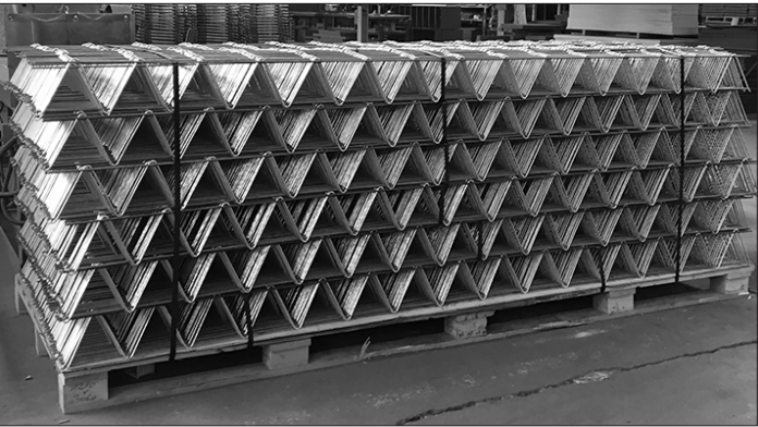
Wire Truss is used to connect the bottom and top concrete layers in a precast “sandwich” panel. Foam insulation is placed between the Wire Truss to create an energy-efficient panel.
