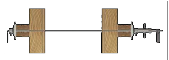
Pencil Rod and Rod Clamps ties formwork together and holds it securely during concrete placement.
