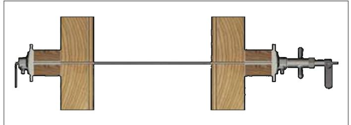
*Pencil Rod and Rod Clamps ties formwork together and holds it securely during concrete placement.*
