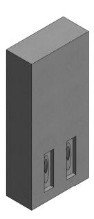
Fill the cavity with grout and finish flush with surface.
