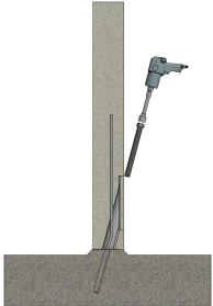
Place a 3/4" x 10" screw anchor though the connector and footing or foundation, then torque to 150 ft-lbs.
