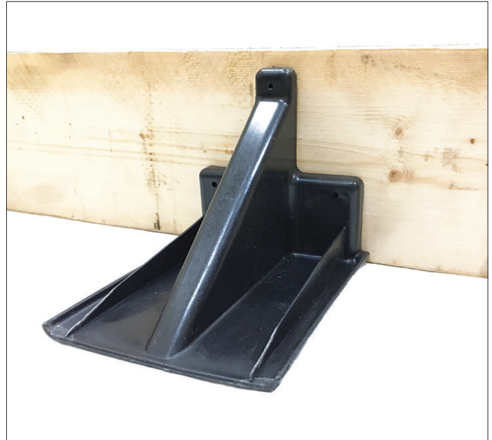
Edge Form Brackets (Type 1) are available in 5" and 7" heights to brace the standard lumber dimensions typically used for tilt-up panel forms.
