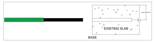
2. Set E2N Square Dowel and Tube in epoxy grout with Tube flush with existing slab and foam on the left and right sides.
