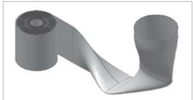
Elephant Trunk controls concrete placement.
