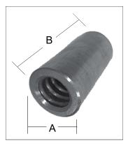
The coil thread is tapped from each side, providing a stop within the center of the coupler.
