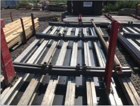
Build and reconfigure the forms you need with the joists or beams you already own.
